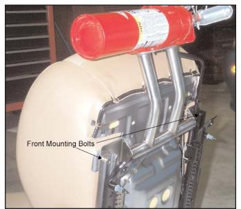
Figure 1.0 - Front Mounting Bolts
