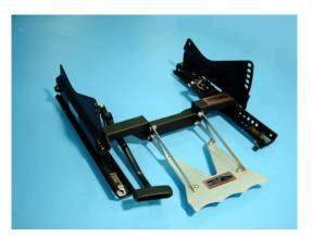
Step 7. Check all fasteners, attach seat to slider/side mount assembly before installing into the vehicle.
