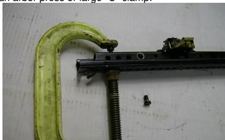
Step 6. Attach the Brey-Krause side mounts to the sliders as shown using factory hardware. (Removable Loctite is recommended). **If also installing Brey-Krause R-9030 anti-submarine strap, begin installation now. If not using Brey Krause R-9030 anti submarine strap mount, insert included spacers between side mount and slider at front.**
