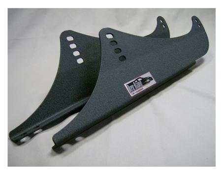
Use the supplied hardware to mount the side mounts to the floor plan.
