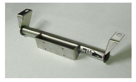
This kit mounts a 2.5 lb quick-release fire extinguisher in front of the driver or passenger seat. The bracket bolts directly to the seat and moves with it, allowing it to accommodate drivers of all sizes.
