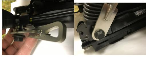
Step 3: Install outboard clip in bracket.
