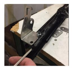
Note: a small portion of cars only have the rear hole in the slider. If your car fall into this category, the second hole must be drilled. We recommend securing slip in belt mount with the first bolt, and using that to locate where the second hole should be drilled. Do not use only one hole to secure the clip in lap belt mount. If the second hole is not centered on the slider, the bolt will not insert.
