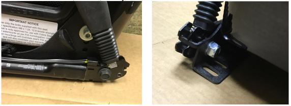
Step 3. Attach side mounts to aftermarket seats, using the hardware included with the seats. It is recommended that you fully tighten the inside (center console side) seat mount to mount bolts, but leave the outside seat mount somewhat loose until installed in the car. Seat height is set by the rear hole, seat tilt is set by the front holes.
