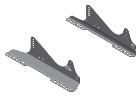
Step 4. Insert seat in car. Forward/back position is set by which holes you choose along the length of the mount. A good starting place is locating the buckle in roughly the same location you noted it was before, in step 1.
