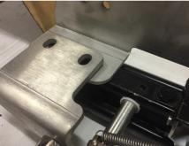
On the outside (door side) slider, the R-9228/9 should be mounted underneath the seat mount (in place of the spacers included with the R-9220/1/2/3 side mounts).
