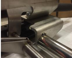
The top of the slider release fingers should be on top of the slider release latch. Use the included springs to maintain contact between finger and mechanism, as well as eliminate vibration. Springs should be used on both fingers.
