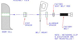
**Note:** Make sure that the bolt threads into the body a depth equal to at least 1 diameter of the bolt. If not, recheck installation.
