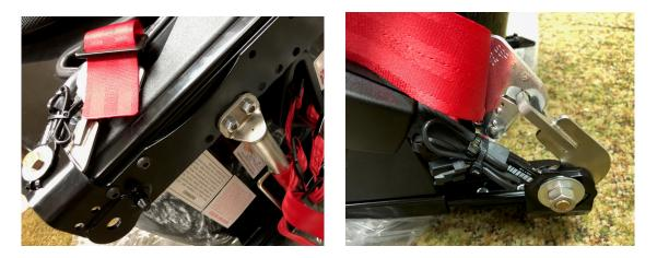
The (included) outboard lap belt mount attaches at the same location as the factory outside lap belt, reusing the stock bolt. If you're also using the R-1150 harness bar, there's no need to install this lap belt mount as the functionality is built into the R-1150's downtube base.
