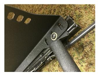
E) Side mounts. The R-9173/4 seat track adaptors are designed to work with either the R-906X line of side mounts (if using Recaro sliders) or the R-907X and R-975X line of side mounts (if bolting the side mount directly to the seat track adapter). The side mounts you use should be selected by the width of the seat you're installing in the car. Use the hardware included with the side mounts to bolt the side mount to the slider or seat track adapter.
