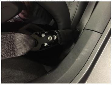
Slide the seat all the way forward and remove the rear torx bolts. Move seat to center position on slider. Lower seat to it's lowest position. Repeat on other seat. Disconnect battery ground cable at the battery. Slide the seat backwards, until the front hooks disengage, then tilt the seat forward. Disconnect seat harness, remove seat from car. Repeat on other seat if doing both seats.
