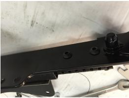
Move slider forward to allow access to lap belt mount area.
