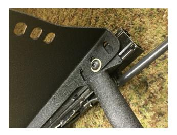
E) Side mounts. The R-9170/1 seat track adaptors are designed to work with either the R-906X line of side mounts (if using Recaro sliders) or the R-907X and R-975X line of side mounts (if bolting the side mount directly to the seat track adapter). The side mounts you use should be selected by the width of the seat you're installing in the car. Use the hardware included with the side mounts to bolt the side mount to the slider or seat track adapter.
