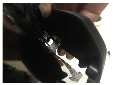
The rest of the cover does not need to be detached to install the harness clips—it can be gently bend out of the way to create the necessary clearance. Use a T50 torx socket to remove the seat belt bolt, insert the lap belt mount outside the factory seat belt, and reattach using the included (longer) bolt and washer. Angle the lap belt mount such that it comes out of the factory rubber seatbelt grommet. Tighten while holding in place.
