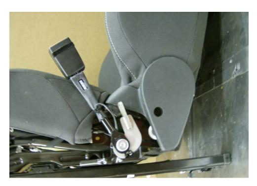
E. Reinstall Seat in car. Note: the lap belt will clip in easiest in the lowered seat position.
