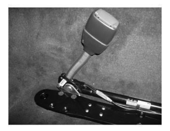
Step 8: Tighten R-9144 down to floor pan with sub-strap mount bar positioned in the desired location. Depending on seat location and belt set-up, choose the most appropriate.
