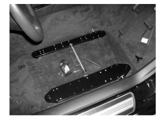
Step 7: Assemble Lap Belt brackets and secure to R-9144 with supplied hardware. Bolt on attachments are recommended for the lap belts due to limited space in the car.
