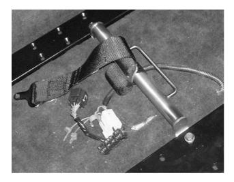
Step 10: Assemble and tighten the outboard lap belt bracket, then mount to the R-9144 with supplied hardware.
