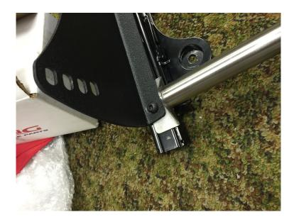
Note: the spacers protruding from the R-9134/9135 face towards the floor of the car. The hollowed out space within is to allow the factory floor mount bolt to recess, so the slider can pass over it.
