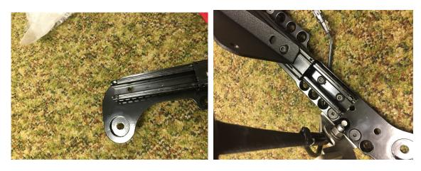
e) Optional: R-2018 Fire Extinguisher Mount The R-2018 fire extinguisher mount goes directly beneath the side mounts, reusing the front mounting bolts on the seat mount. If using a Recaro slider, this means the R-2018 is inserted between the slider and seat mount.
