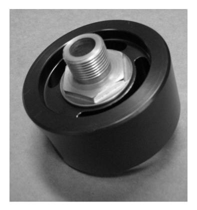
Step 4: Install the new oil filter to the R-9096 unit by threading it onto the threaded fitting. On 968 engines, some mild filing may be needed on the timing cover due to slight contact.
