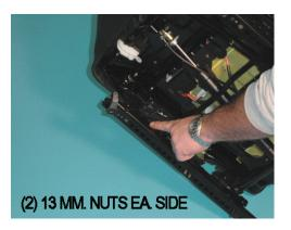
Step 5. Attach the Brey-Krause side mounts to the sliders as shown using factory hardware. (Removable Loctite is recommended). If also installing Brey-Krause R-9030 anti-submarine strap, begin installation now.
