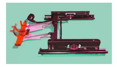
Step 6. Check all fasteners, attach seat to slider/side mount assembly before installing into the vehicle. (Install supplied shims under back of R-9091 bracket if mounting optional R-9030 anti-sub strap under front of R-9091 bracket.)
