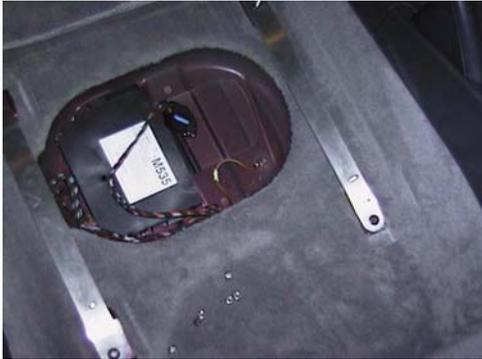
Step 3. Determine the desired fore/aft seat position by placing seat with R-908X series side mounts onto adapters.
