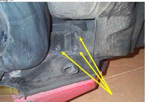
Locate the three nuts located on the inside of the rear quarter panel.
