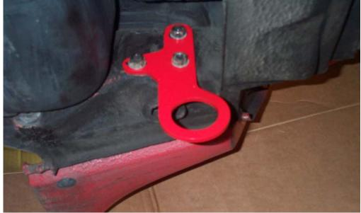
Remove nuts. Install bracket as shown. Note: You may want to apply some sealer around the studs to prevent water leaking into the trunk. Install and tighten nuts.
