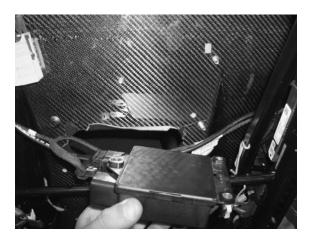
Step 5: Install the black box relocation tab on the lower most bolt, lightly tighten with it positioned towards the front of the seat.
