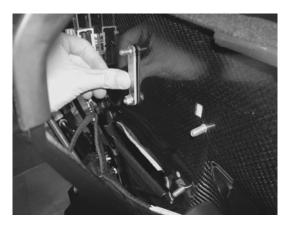
Step 6: Position the black box on the tab's stud and upper right most stud so that the box's orientation is like that shown below. Cutting of the one or more zip ties may be necessary. Tighten all three bolts, and tighten the supplied flange nut for the tab stud.
