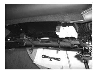
Step 5: Wrap the sub-strap belt to the appropriate length and through its 3 pass locking plate (supplied from belt manufacturer).
