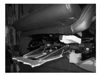
Step 7: Reinstall the seat and secure it with the factory floor pan bolts.
