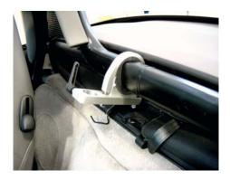
Slide upper portion of mount into lower portion as shown,
