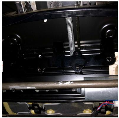
Outer holes (in boxes) are mount points for the BMW release bracket/fire extinguisher. The inside holes (circled) are for a standard Amerex fire extinguisher bolt pattern (which is also what the Brey Krause quick release handle uses).
