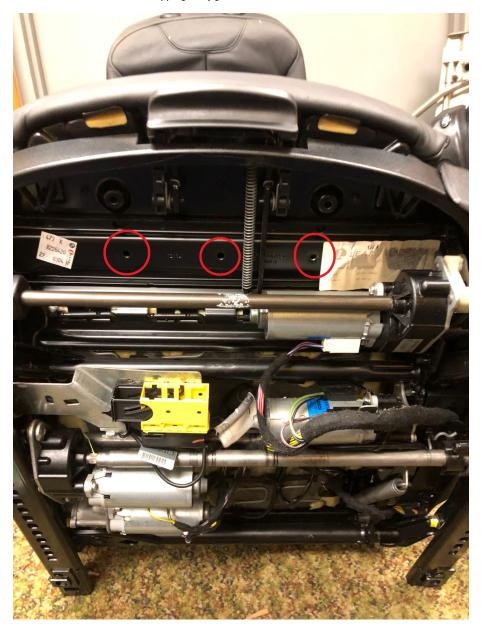
First insert all bolts a couple turns. Be careful of angle as you are tapping the holes at this point. Once all bolts are inserted a couple turns, tighten until snug, 15 ft lbs. Over tightening will result in stripped holes.
