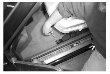
Step 2. Remove nuts. (Both inside and outside tracks).
