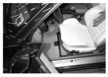
Step 5. Position extinguisher bracket as shown and attach using supplied hardware.
