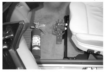
Step 6. Carefully move seat forward making sure that there is no interference between the extinguisher/mount and the seat. Pay special attention when the seat is in the foremost position, making sure that the front of the seat does not contact the extinguisher.
