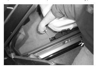
Step 2. Remove nuts. (Both inside and outside tracks).
