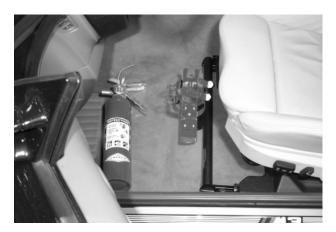
Step 6. Carefully move seat forward making sure that there is no interference between the extinguisher/mount and the seat. Pay special attention when the seat is in the foremost position, making sure that the front of the seat does not contact the extinguisher.
