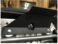
Step 5. Set seat upright, attach fire extinguisher mount of choice. Reinstall seat in car, making sure not to reconnect battery until seat wiring harness is reconnected.
