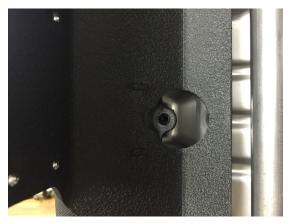
Step 4. Tighten down large bolts, ~12 ft lbs. Tighten small bolt until snug, but not tight (this bolt is just for locating, not supporting-- over tightening will strip the screw clip).
