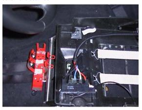
Step 4. Reinstall two front seat bottom to seat track-mounting bolts and tighten the rear seat bottom to seat track bolts.
