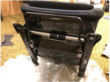
Step 5: If using R-2295 fire extinguisher mount, attach it at the location marked below now.
