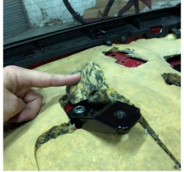
4. Install smaller inside mount. The smaller inside mount attaches to the center LATCH point. In order to make this strong enough for harness use, a high strength bolt is provided, as well as a load spreading aluminum plate that gets mounted inside the trunk. **Do not reuse the stock hardware at this location!** Secure the small mount using the include bolt. This is the passenger's inboard mount.
