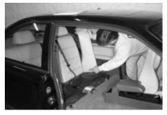
Step 3. Remove rear inside 1/4 panels carefully - pop out.
