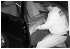
Step 2. Remove outside seat back cushions. Carefully pull at top rear edge, rotate & pivot to clear lower pivot pin.
