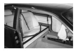
Step 10. Carefully remove the plastic cover at lower shoulder strap mounting point located along the doorsill to expose the mounting bolt.
