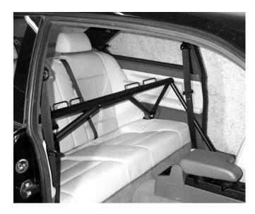
Note: Belts are to be wrap mounted around the main tube.
