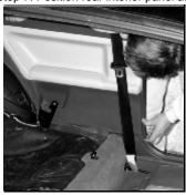
Step 8. Reverse steps (1-2) to reassemble interior panel as shown below. **Tip:** Use a small phillips screwdriver to reposition the rubber gasket over rear interior panel as shown below.
