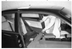
Step 4. Remove outside rear seat belt buckle, mounting bolt and washers.
