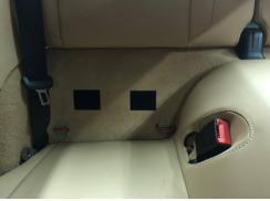
d. Remove the rear lower seat cushion. To do so, first pull up the outside of the seat on both sides (secured by Velcro). Next lift the rear middle of the seat, sliding the entire seat rearwards and the seat back upward. This will release two slotted mounting tabs towards the front of the seat cushion.
