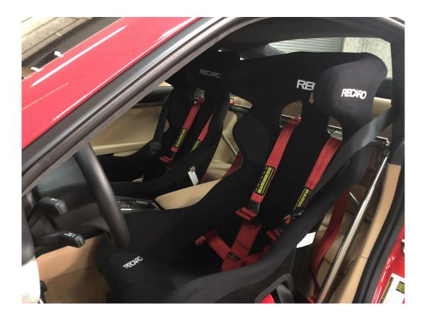
Note: Periodically recheck fasteners for tightness. Shoulder straps should be wrap mounted around main tube and thru guides.
