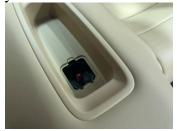
b. Remove the trim covering the inboard seatbelt receiver mount nuts, remove the nuts, remove the seat belt receivers:
