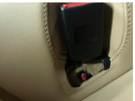
c. Remove the rear seat lower seat back support. This is just held on by Velcro, so removing just consists of pulling it off:
